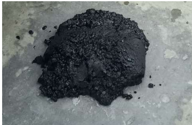
Figure 4. 3 Fresh SCBA-Based GPC
