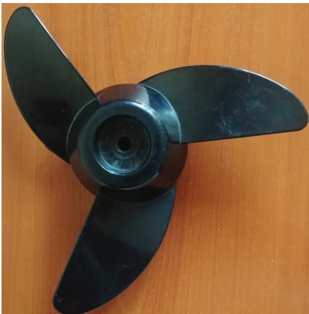
Figure 1. 240 mm diameter 3-swept-back rotor blade.
