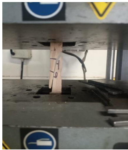
Figure 5: Failure During Laboratory Tensile Test
