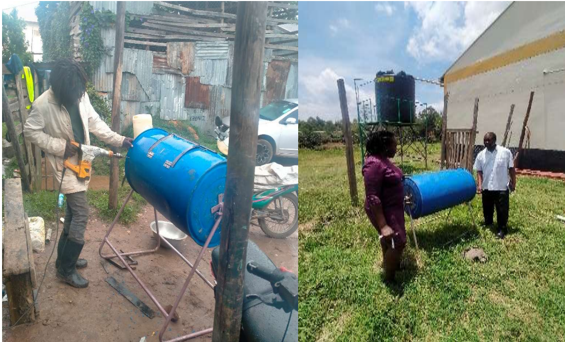
Plate 9: Picture showing a fabricated composting bin (blue drum) (Source, author, 2021)
