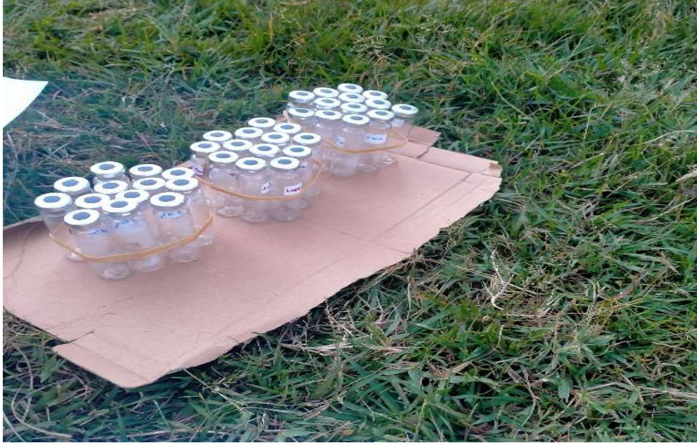
Plate 4: Glass vials fitted with rubber seal for holding GHGs (Source, author, 2021)
