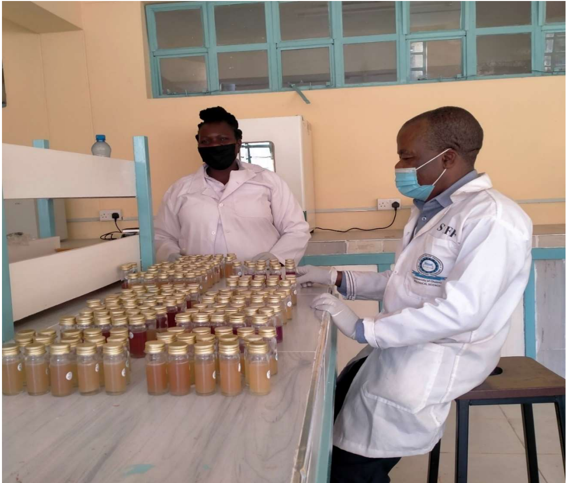
Plate 7: Serial dilution of pond water samples before culturing of bacteria (Source, author, 2021)
