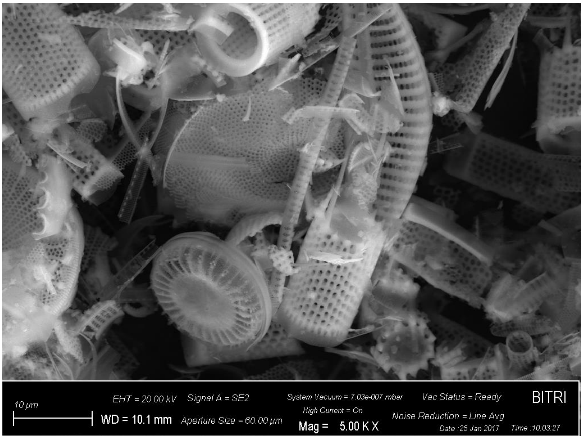
Figure 4.4 (a): SEM micrograph of unmodified diatomaceous earth (DTE)
