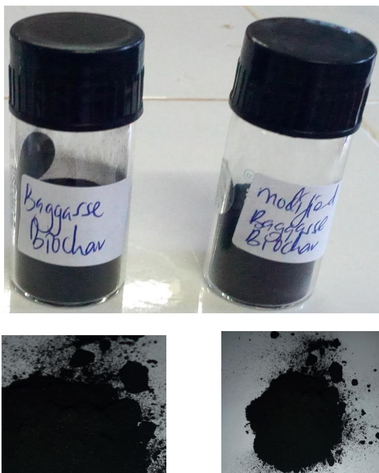
Figure 3.2: Photograph showing unmodified bagasse biochar (CBG) and iron modified bagasse \alpha -Fe 2 O 3 -CBG adsorbents
