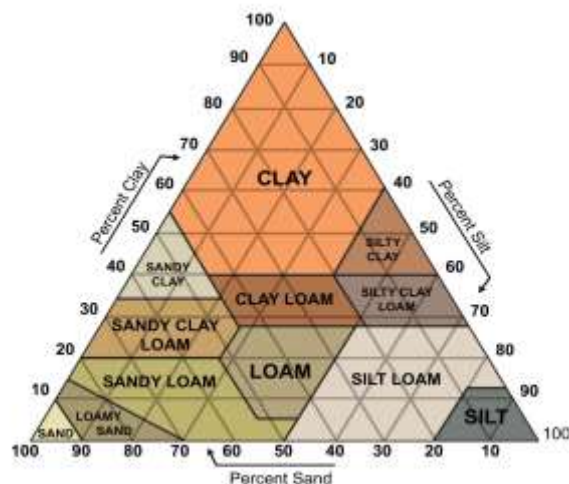
Figure 3.2. The soil textural triangle can be used to classify soils according to their particle size distribution (Okalebo et al. 2002).
