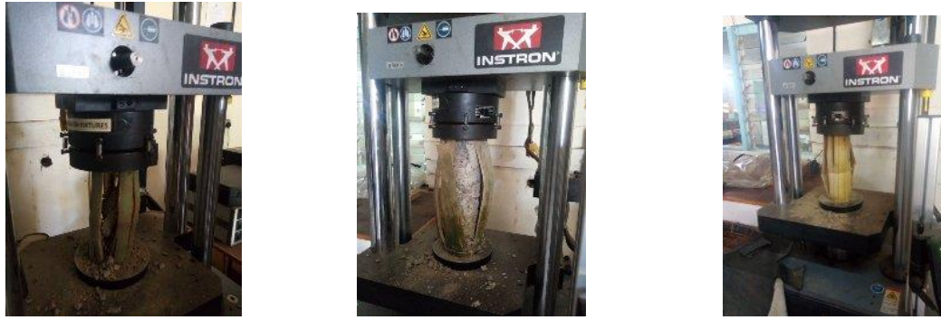
a) Bamboo filled with C20 b) Bamboo filled with C30 c) Raw Bamboo
