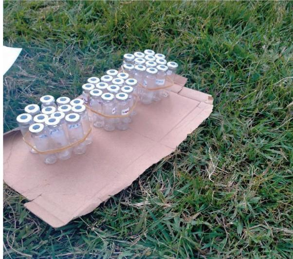
FIGURE 2: Glass vials fitted with a rubber seal for taking gases to the laboratory for analysis.
